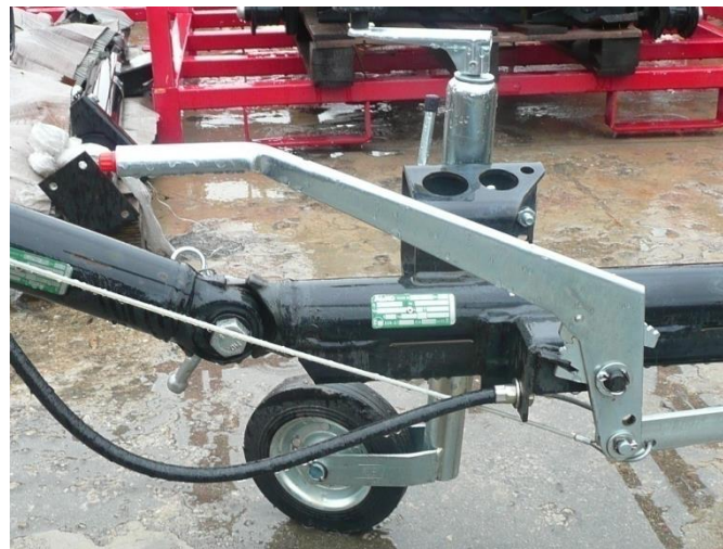
Figure6.4-2 Lever of the manual park brake with release red push-button
